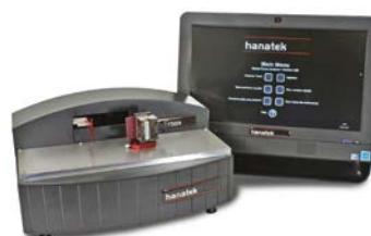
Carton Force Analyser For more repeatable testing and the ability to test small samples.
